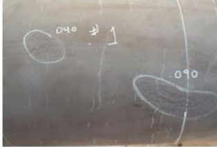
Defect - External Wall Loss
